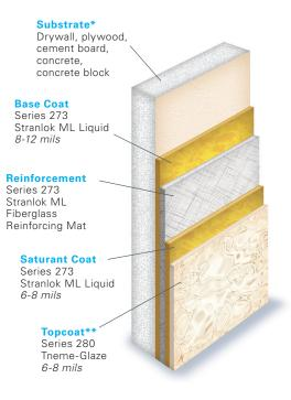
\*A variety of fillers and surfacers are available depending on substrate, including Series 215 Surfacing Epoxy and Series 130 Envirofill for use on concrete block. Contact your Tnemec coating consultant for recommendations.
